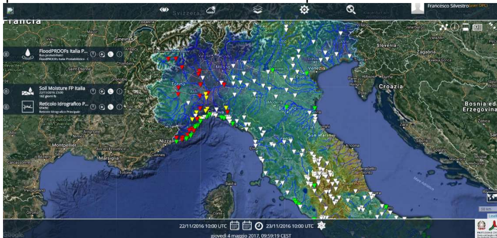
Figure 2: Event on 23/11/2016; flood forecasting chain. Control sections coloured basing on the overcoming of predefined thresholds. Soil Moisture Map (root-zone) is also shown
